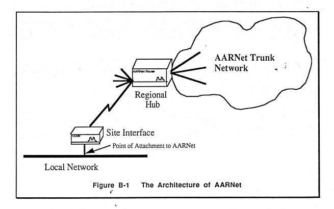
This architecture is very effective, due to its underlying simplicity and flexibility. The interconnection of the routers can be implemented by any reliable digital transmission medium, including low and high speed leased lines, switched circuits (such as ISDN or
